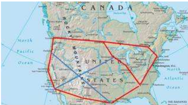
Figure 3: North American HVDC Hybrid Grid Concept (red lines are elpipes, blue lines are 800kV HTS lines)
