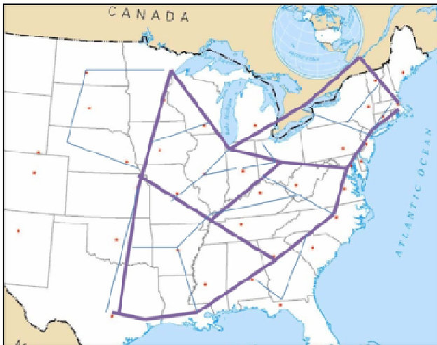
Figure 5: HVDC Grid for Eastern US
